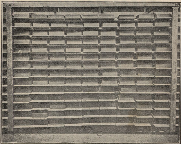
FIG. 3,822.—Sub-section of Lancaster "Martin" steam pipe rack brick dryer. The section is 8 ft. between centers of supporting racks, 14 shelves of pipe in height, 5 ins. center to center of pipes, 9 pallets of brick in width. The sub-section holds 126 six brick pallets of bricks or 756 bricks.
