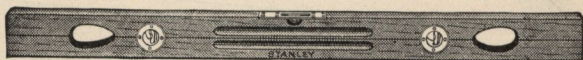
FIG. 3,919.—Stanley light wood adjustable mason's spirit level and plumb rule, with double plumb opening for bob.
