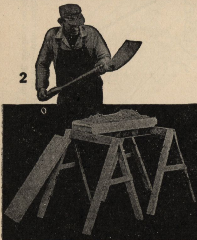
FIGS. 3,783 TO 3,786.—Raber and Lang hand mould for concrete brick, illustrating method of use. Fig. 3,783, filling mould with material; fig. 3,784, tamping with shovel; fig. 3,785; rocking over; fig. 3,786, releasing finished brick. Average time to make 6 bricks, 36 seconds.
