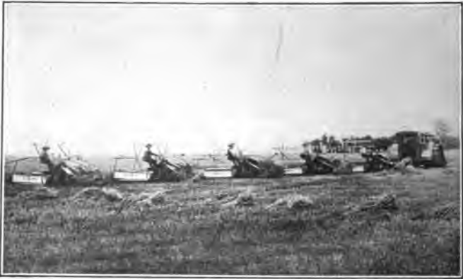
MODERN OIL TRACTOR OPERATING FIVE BINDERS
