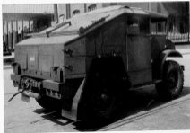
FIGURE 105.—Morris CA tracked field artillery tractor (model of type).
