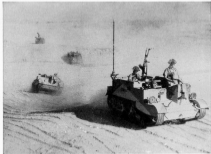
FIGURE 31.—Universal powered carrier fitted with 30-cal gun on anti-aircraft mount and with Boys anti-tank rifle.
