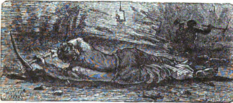
"HOLING COAL."—The collier, lying on his side, with his neck bent in a most painful position, makes an horizontal cut with his pick at the bottom of the seam.
