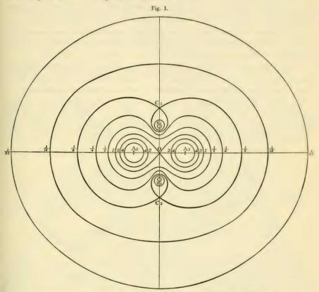
I have produced these curves in the jelly of isinglass described in Case I. They are best seen by using circularly polarized light, as the curves are then seen without interruption, and their resemblance to the calculated curves is more apparent. To avoid crowding the curves toward the centre of the figure, I have taken the values of I for the different curves, not in an arithmetical, but in a geometrical progression, ascending by powers of 2.
