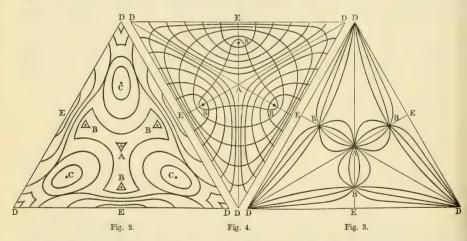
The lines of equal intensity of the action on light are seen without interruption, by using circularly polarized light. They are represented in Fig. 2, where A, BBB, DDD are the neutral points, or points of no action on light, and CCC, EEE are the points where that action is greatest; and the intensity
