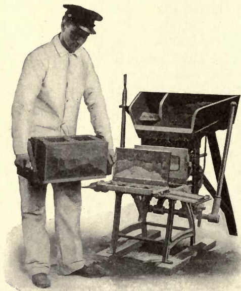
FIG. 17—A Machine for Making Hollow Concrete Blocks.
