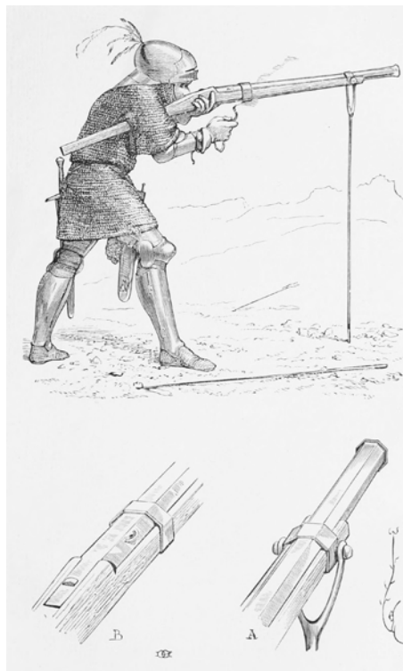
Depiction of an arquebus fired from a fork rest. Image produced in 1876. (Public Domain)
