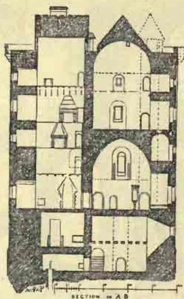
FIG. 299.—Borthwick Castle. Transverse Section through Hall.
