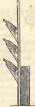
Fig. 29. SECTION SHOWING SIDE OF GRAPE-ROOM AT HECKFIELD WITH THE MODE OF ARRANGING AND FIXING THE BOTTLES. (From Parks and Gardens of Paris .)
