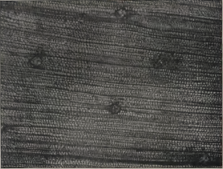
Transverse Section of Creosoted Scots Pine Wood-paving Block (Bethellised). The blurred appearance is due to the creosote pressed into the tissue. The medullary rays and the resin-ducts are completely filled with creosote and resin.
