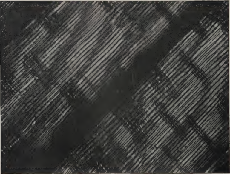
Longitudinal Radial Section of same Block. Showing the tissue, the medullary rays (filled with creosote), the autumn zone, and the bordered pits peculiar to the wood of the Pine.
