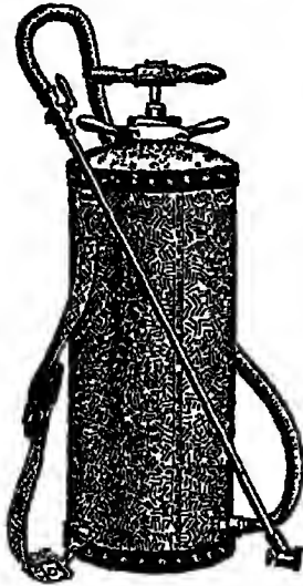
Fig 79 Air pressure sprayer: Galvanized iron tank. Brass is far better because resistant to spray chemicals
