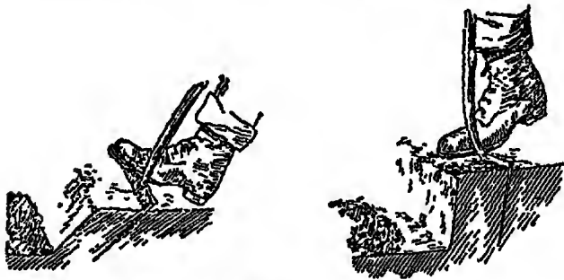
Fig 46 Wrong and right ways to dig
