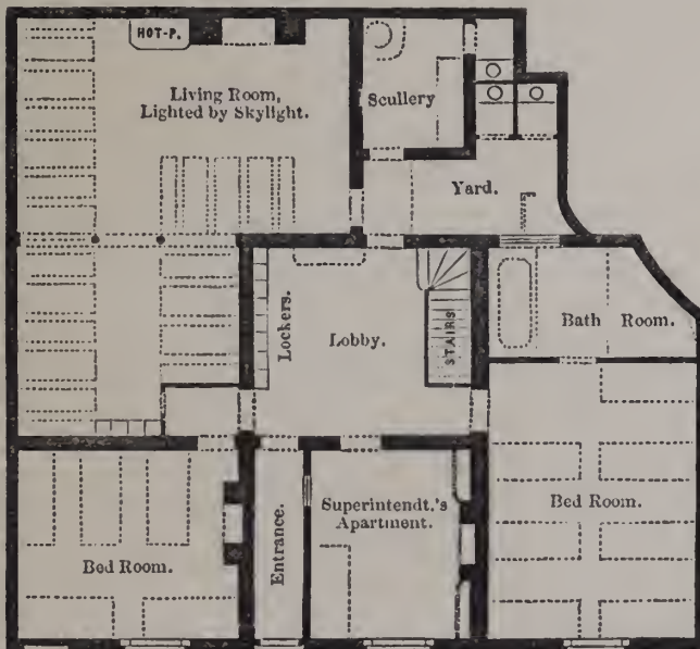
Ground-Floor Plan of the Renovated Lodging-House, Charles-street, Drury-lane, to accommodate 82 Single Men.
