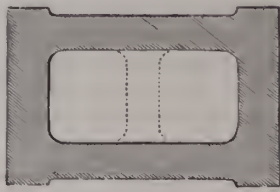
Section (1/4 full size) of a Hollow Brick adapted for Floor Arches, &c.
