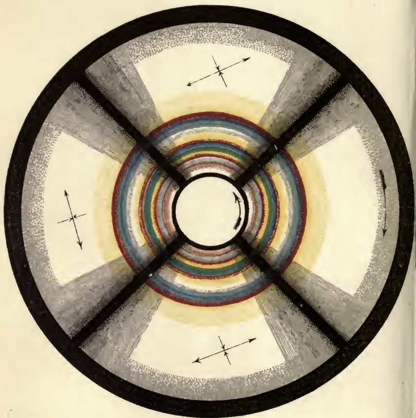
DIAGRAM SHEWING THE COLOURS EXHIBITED BY A PLATE OF GELATINE WHEN EXPOSED TO A TORSIONAL SHEAR.
