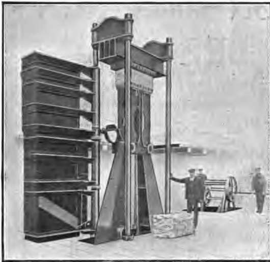
Hand Press supplied to the Government of India for use in a Jail. Box 12ft. deep, bale 200lbs., 8½ cubic ft.
